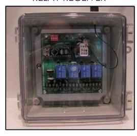
The WXL Series Receiver features up to 4 control relays. The unit also provides an Alarm output for Transmitter low power or RF signal loss.
