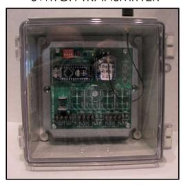
The WXL Series Switch Transmitter features up to 4 dry-contact inputs that activate relays of the receiver unit. The unit also sends supervisory system data to the receiver
