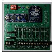
The WXL-ME Series Switch Transmitter features up to 4 dry-contact inputs that activate relays of the receiver unit. The unit also sends supervisory system data to the receiver
