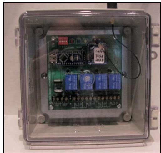
The WXL Series Receiver features up to 4 control relays. The unit also provides an Alarm output for Transmitter low power or RF signal loss.
