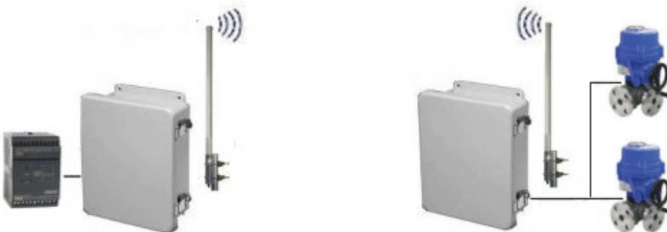
PLC controlling two different irrigation valves up to 10 miles away.
