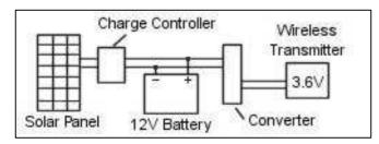
Application example using Model: PCM2-3.6
